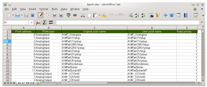
By modifying **User Point name** (column D) you can change the name of point on export to Bacnet. **Priority** (column E) defines reading priority. If priority is set to 0, point will not be exported to Bacnet and its reading will be disabled. If priority is set to value greater than 0, on every reading the value decrements and if resulting value is 0, point value will be read and priority value will be set back to original value defined in xlsx file.
